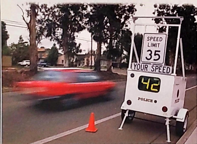
Figure 11 A speed-monitoring trailer uses radar to measure the speed of an approaching car. It reminds motorists of the posted speed limit and makes them aware of their actual speed.
